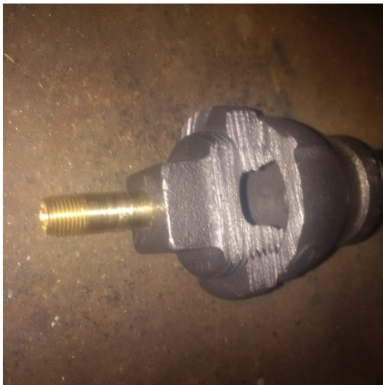
The cut section of the burner and fitting of the nipple
