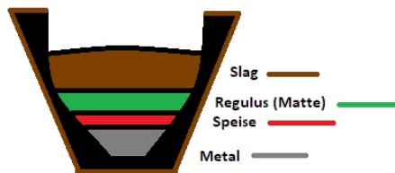
Crucible with contents layered after fusion
